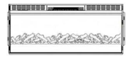
5. Once completed installing crystal embers or fire log, reinstall glass panel. The hooks on the back of the glass panels fit into the slots on the side of the firebox. Once in the slots, the glass panel goes down and locks into place. Once in place, reinstall 2 locking screws to hold glass securely in place.
