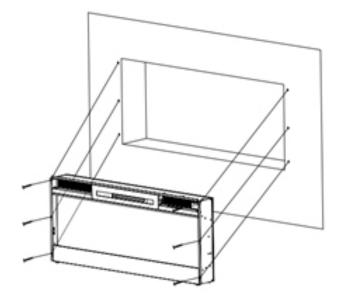
4. Once the fireplace is installed in the wall, place crystal embers or fire log in the fireplace.
