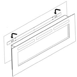
Mounting bracket installed on wall
