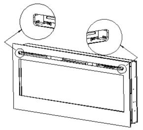
2. After removing screws, lift glass panel UP and STRAIGHT OUT toward you to remove from fireplace. Place glass panel in a soft, dry place.
