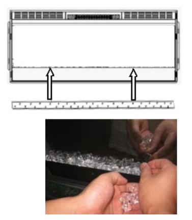
2. Carefully, place crystal embers on plastic strip as illustrated in the picture to the right. Apply an even layer from side to side.
